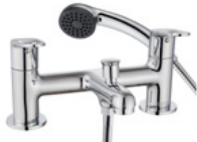
Bath Shower Mixer IRS BSM C PW NB Spout projection 112mm Long life 1/4 turn ceramic disc valves for added durability and smooth control. Robust metal fixing nut to secure the tap in place reducing the risk of loosening over time. A hard-wearing, flawless, scratch resistant chrome finish that lasts for years.
