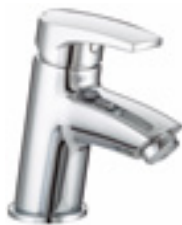
Basin Mixer with Clicker Waste OR BAS C PW NB Spout projection 94mm Fitted with a flow regulator, limiting the flow of water to 5 litres per minute, reducing the amount of water used. Long life ceramic cartridge for added durability and smooth control. A hard-wearing, flawless, scratch resistant chrome finish that lasts for years
