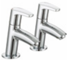
Basin Taps OR 1/2 C PW NB Spout projection 82mm Long life 1/4 turn ceramic disc valves for added durability and smooth control. Robust metal fixing nut to secure the tap in place reducing the risk of loosening over time. A hard-wearing, flawless, scratch resistant chrome finish that lasts for years
