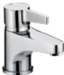
Basin Mixer with Clicker Waste DUL BAS C PW NB Spout projection 75mm Long life ceramic cartridge for added durability and smooth control. A hard-wearing, flawless, scratch resistant chrome finish that lasts for years
