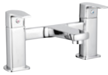
Bath Filler NVA BF C PW NB Spout projection 95mm Long life 1/4 turn ceramic disc valves for added durability and smooth control. Robust metal fixing nut to secure the tap in place reducing the risk of loosening over time. A hard-wearing, flawless, scratch resistant chrome finish that lasts for years
