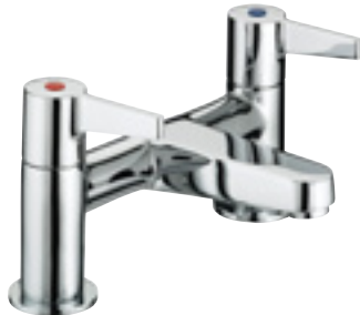
Bath Filler DUL BF C PW NB Spout projection 110mm Long life 1/4 turn ceramic disc valves for added durability and smooth control. Robust metal fixing nut to secure the tap in place reducing the risk of loosening over time. A hard-wearing, flawless, scratch resistant chrome finish that lasts for years
